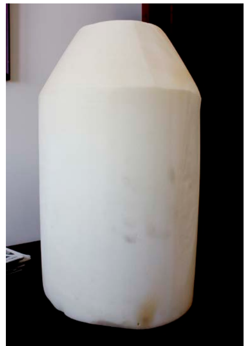
A swab similar to this one will be pushed through the water line between the North Tyndal wellfield and the reservoir on Willow Street on June 4 as the town begins its annual flushing of the water lines. (Town of Amherst photo)
