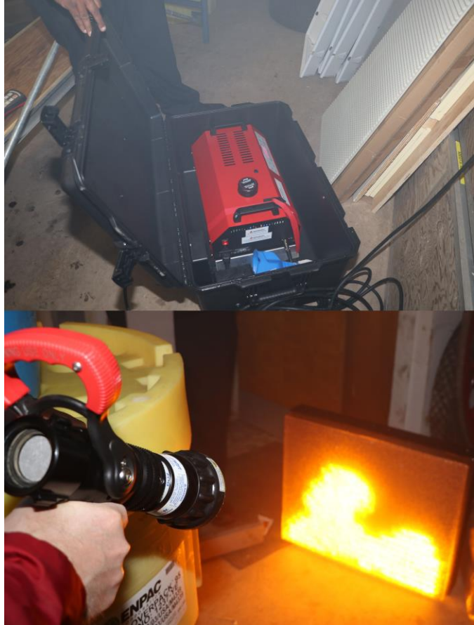
The parts of the fire simulator recently obtained by the Amherst Fire Department include the smoke machine (top picture), an electronic nozzle and a digital simulation panel. (Tom McCoag / Town of Amherst)
